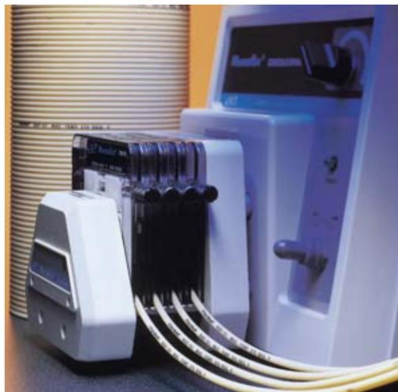
Pharmed® (TBG007) tubing is a clean , flexible tube that is compatible with peristaltic pumps.
