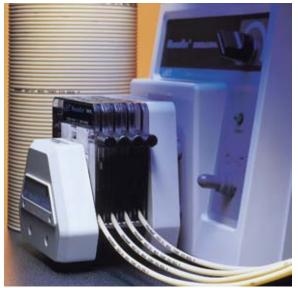
Pharmed® (TBG007) tubing is a clean , flexible tube that is compatible with peristaltic pumps.
